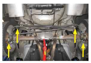
8. Remove the four 15mm nuts from the bushing brackets at the ends of the original sway bar.
